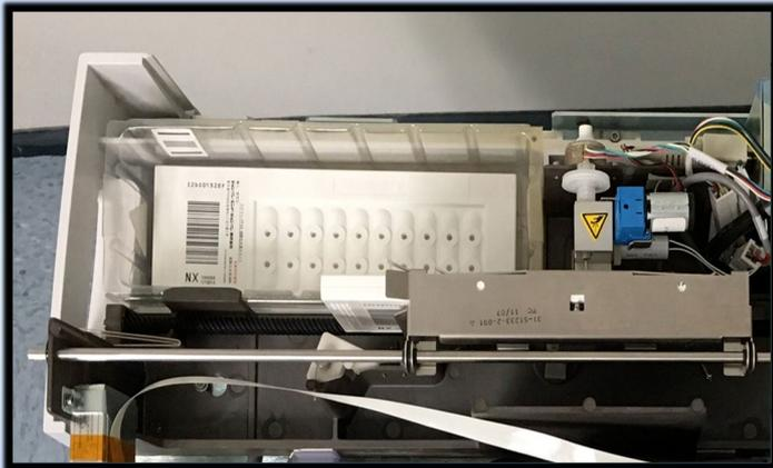
The Hydrogen Peroxide Delivery Assembly moves hydrogen peroxide solution from the Cassette Assembly to the Vaporizer Assembly.
