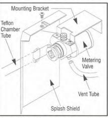
The new RPI metering valve to fit the Chemiclave has a splash shield to prevent exhaust fluid from spraying into other areas of the machine - it's added protection.
