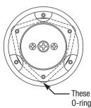
When replacing the O-ring ensure that it is routed in and out of the pins as shown.
