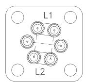
**NOTE:** For 6500 WATT operation, only 2 jumpers are used. Note the location of the L1 and L2 connection points.
