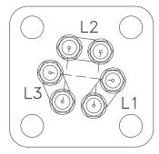
**NOTE:** For Three Phase, 9750 WATT operation, only 3 jumpers are used. Note the location of the L1, L2 and L3 connection points
