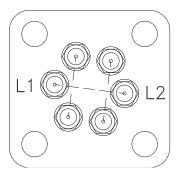
**NOTE:** For 3250 WATT operation, no jumpers are used. Note the location of the L1 and L2 connection points.
