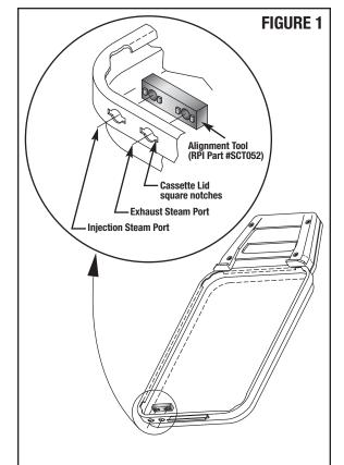
Angle cassette lid as shown, using gravity to aid in tool positioning while assembling and closing the cassette.
