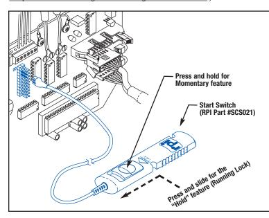
TIP - To guide the Start Switch Connector to Pins #18 and #16, start at the pin labeled "20", count down one pin, which is Pin #18, then count down one more pin, which is Pin #16. Gently guide the Start Switch Connector to both Pin #18 and #16, leaving all other pins exposed.
