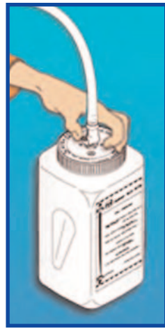
RPI's unique design includes a "quick disconnect" that allows the Condenser Waste Bottle to detach from the unit with just a simple snap.
